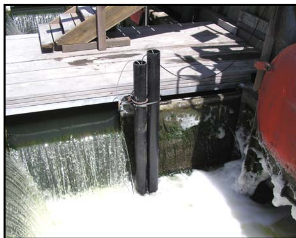
Figure 2-1: Datasonde holder within Weir Structure
